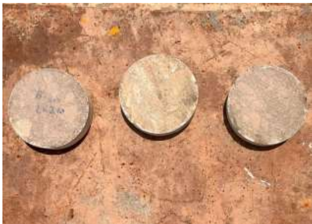
Figure 3. Sample examined for RCPT
